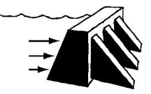
Water pushes against this dam but the dam pushes back against the water. This prevents the dam from falling over. The weight of the dam also pushes downward as well.
